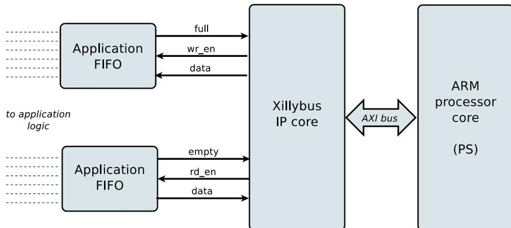
As shown above, the application logic on the FPGA only needs to interact with standard FIFOs.
