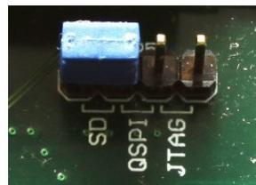
The other jumpers are set depending on the desired operating mode. For example, the power supply jumper can be set to take power from an external 5V source, or from the UART USB jack – both are fine for a successful boot of Xilinx.
